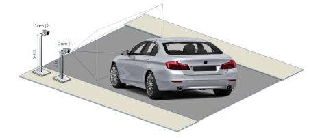
• **For Highway:** Height of Installation of the Camera is variable and can go up to 25 feet. The angle of Incidence should be between 10 to 40 degrees.
