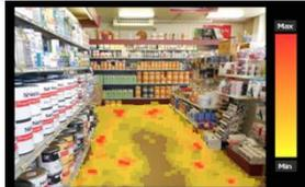
Object movement density represented with color gradient over the monitored area or specified region of interest based on specified time duration.
