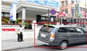
Detects parking or stopping by any vehicle in a specified virtual area (no parking zone or restricted zone) beyond a specified period.
