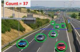
Counting of vehicles that cross a virtual line in a vehicle lane or entry / exit gates.
