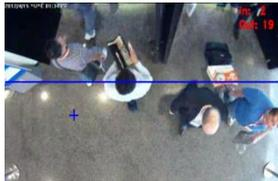
Counts the number of people traversing a certain passage. While angular camera can also be used, best results are achieved with head detection in overhead camera at entry / exit. Counts are provided in both directions (coming in/going out)
